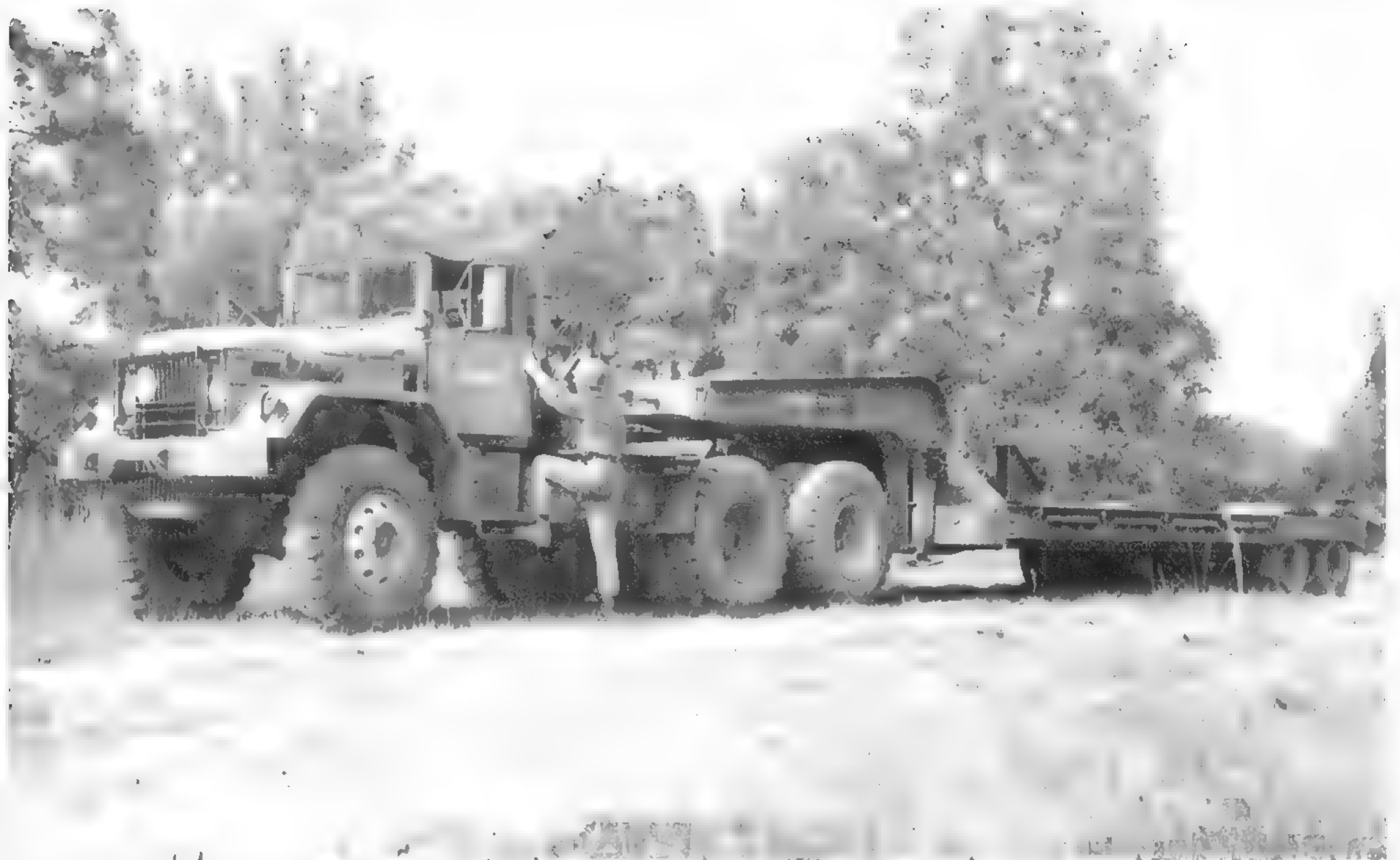
This M123 was coupled to a M162 60-ton lowboy for an October 1961 photo. It has had a siren added to it. The relocation of the towing shackles on the front bumper may have been an effort to resolve compatibility issues with the military standard 5-ton wreckers. Ultimately, towing these trucks with the standard wreckers was prohibited. The front wheels on this truck are non-standard. (U.S. Army photo)
